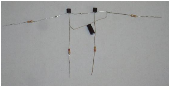
First Capacitor Placement
