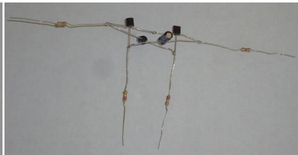
Second Capacitor Soldered
